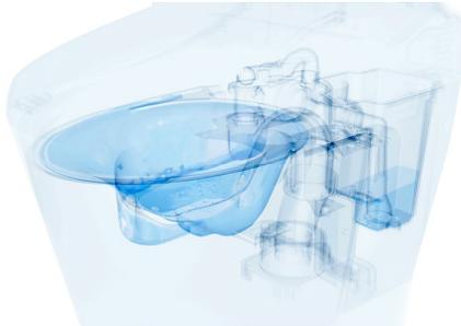
TOTO's Ultra High-Efficiency Tornado Dual-Flush System employs a reserve water tank and pumping system inside the toilet that combines with the home's direct water supply to realize its 1.0-gpf / 0.8-gpf flushing capability. To achieve this, TOTO engineers designed a revolutionary flushing system in which the siphon jet is fed from water that is pumped into the bottom of the bowl from the reserve tank, while the powerful rim and bowl wash is supplied directly by the home's water supply.
