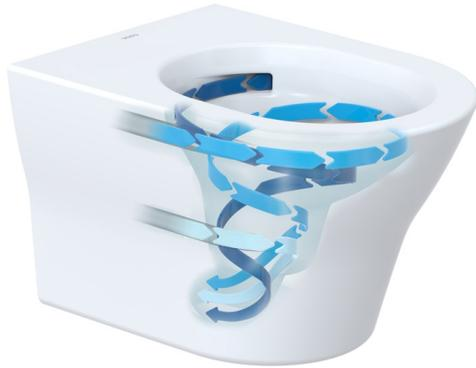
Inspired by tornados in nature, TOTO engineers harnessed the power of gravity and water to spin away waste by designing a seamless bowl interior with a concave rim to channel high-speed water jets. Each flush effectively removes matter, debris, stains, residue, and limescale, as it provides superior bowl and rim cleansing action.
